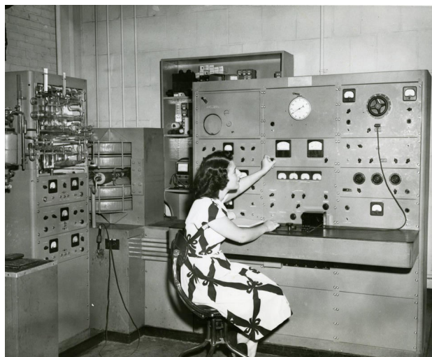
Credit: NIST In this 1948 photo, a NIST staff member operates an early mass spectrometer.
